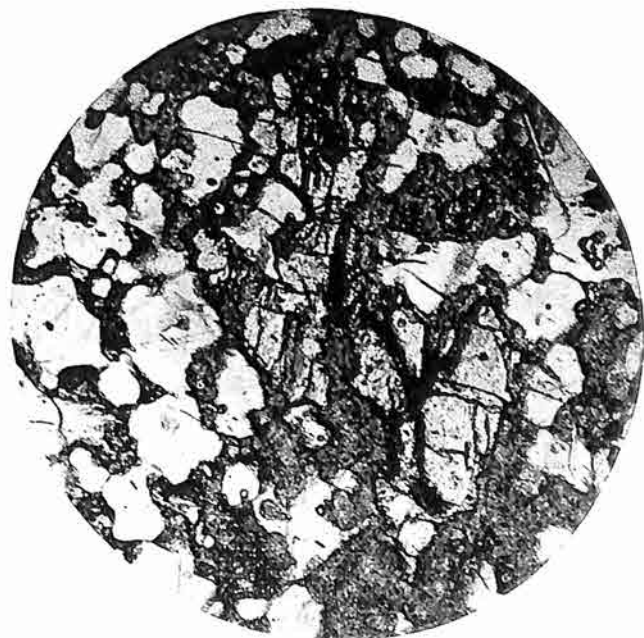
Fig. 5. Andalusite (showing cross-fractures) and serrate in andalusite hornfels. \times 34 (V. 1137).
