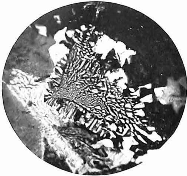
Fig. 1. Granophyre of quartz and potash feldspar in quartz diabase. Crossed Nicols. \times 105 . (V. 241).
