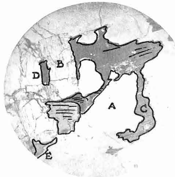
Fig. 6. Corroded (?) biotite crystal in biotite granite. Crossed Nicols. \times 22 , \lambda , 52.
