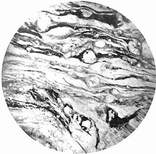
Fig. 1. Mylonized part of cataclastic granitic-gneiss, showing pseudo-fluidal texture. \times 20 , (V, 324).
