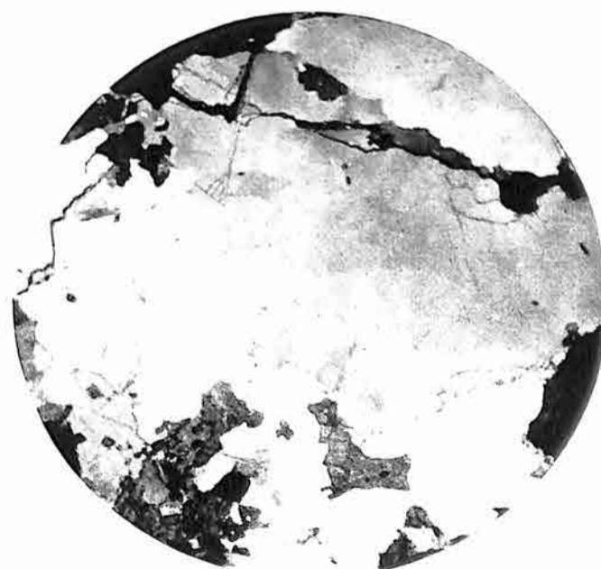
Fig. 5. Undulose quartz, in part crushed, in granite. Crossed Nicols. \times 25 . (Y. 116).
