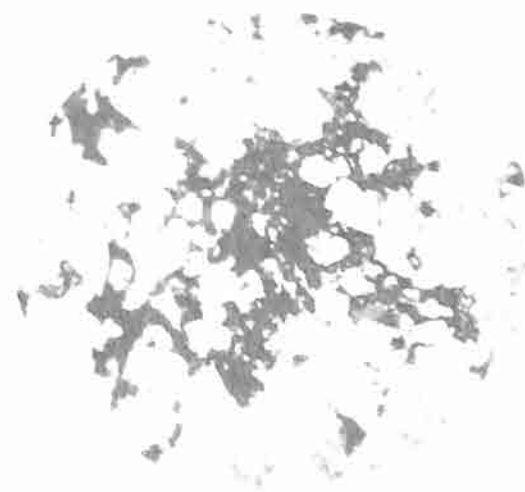
Fig. 4. Small hornblende crystals in hornblende granite, 100 μ (X 175).
