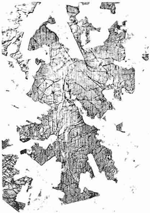
Fig. 2. Monoelinic pyroxene dissected at the edges by smaller and idiomorphic plagioclases in quartz gabbro, \times 27 , (Y, 216).
