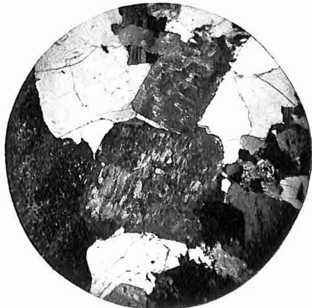
Fig. 5. Idiomorphic potash feldspar in biotite granite. Crossed Nicols. (V. 203).
