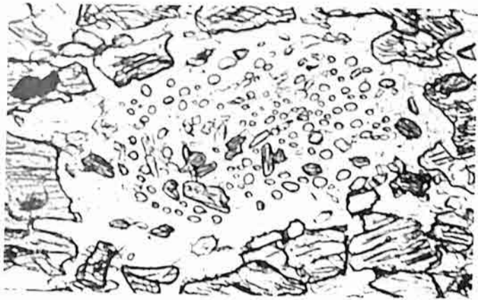
Fig. 1. Crystalloblastic plagioclase enclosing numerous quartz-droplets in hornblende gneiss. \times 60 . (V, 174).
