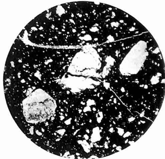
Fig. 4. Fragments of crushed feldspar and quartz enclosed in pseudo-tachylyte. \times 31 , (V, 324 B.).
