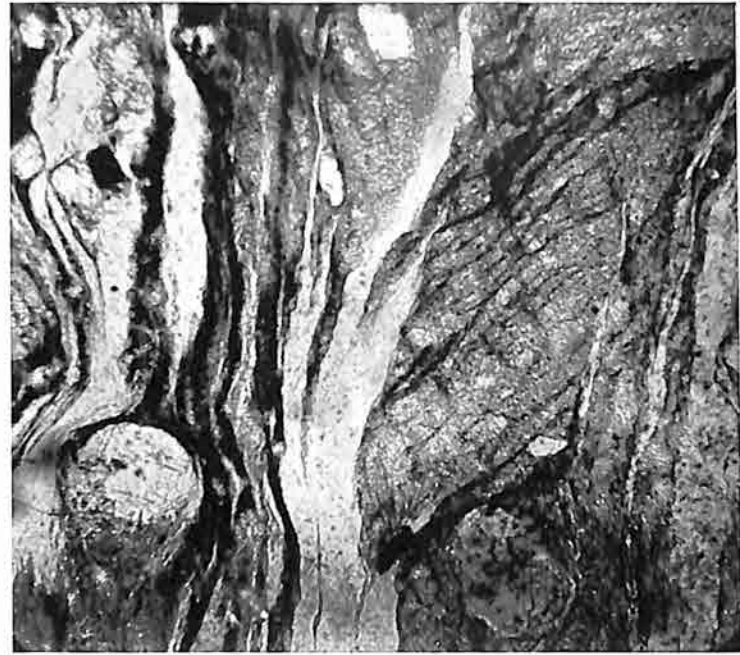
Fig. 2. Detail of mylonitic part of eye-gneiss showing rolled out quartz streaks. Crossed Nicols. \times 40 . (Y. 324).
