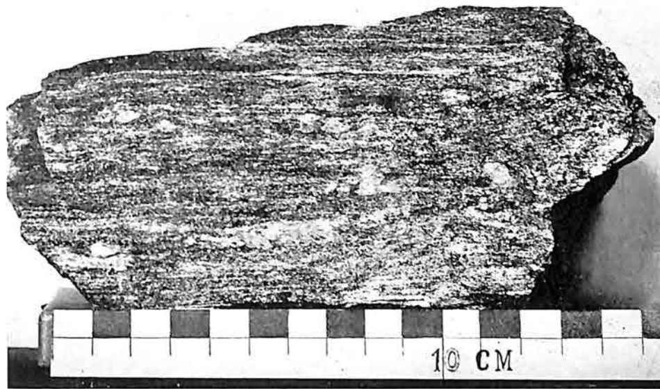
Fig. 1. Biotite granite-gneiss showing distinct parallel texture. King Frederick William IV fall, Courantyne. (Y. 270).
