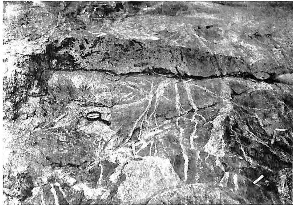
Fig. 3. Dark diorite-gneisses intruded by network of light coloured diorite-aplite, Mamma dam ( = Sisabo fall) Suriname river.
