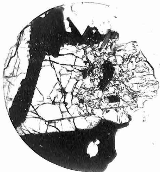
Fig. 5. Primary epidote encrusted with fine-grained colorless minerals; in quartz mica hornblende diorite; \times 110 . (X, 14)
