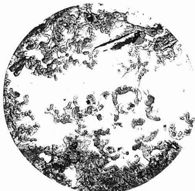
Fig. 4. Quartz containing curved chlorite aggregates. \times 72 . (Y. 601).
