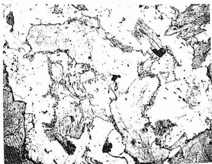
Fig. 3. Epidioritised gabbro showing secondary hornblende. \times 19 . (V. 5090).
