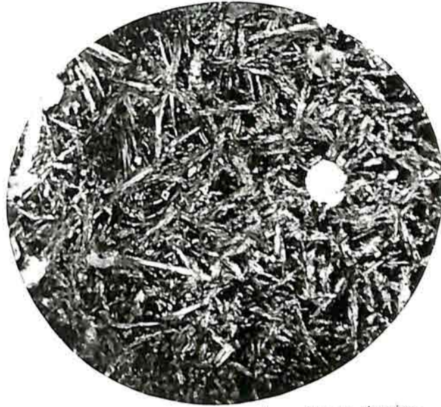
Fig. 2. Groundmass in hypersthene diabase showing split plagioclases. Crossed Nicols. \times 25 . (V. 70).
