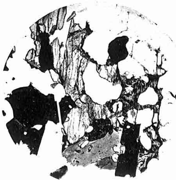
Fig. 5. Corroded monoclinic pyroxene (left) and orthorhombic pyroxene (right) in biotite granite. \times 30 . (Y. 107 B).
