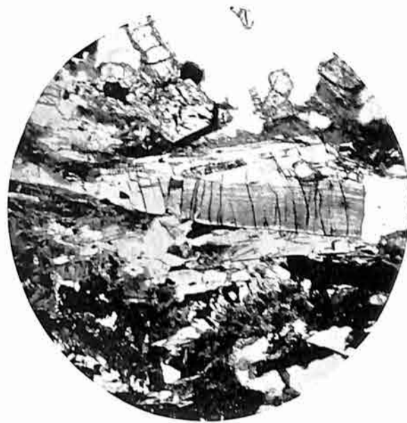
Fig. 2. Large sillimanite-needles with cross-factures and enclosed dust; in sillimanite-hypersthene gneiss. \times 11. (V. 2064).
