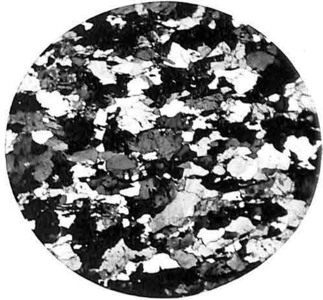
Fig. 2. Quartz mica diorite-gneiss, "irregular" structure-type, Crossed Nicols, \times 17 . (V. 483).
