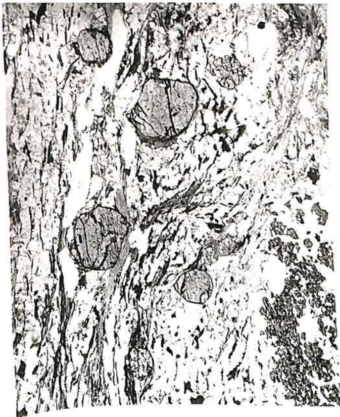
Fig. 3. Porphyroblasts of garnet and skeleton of staurolite (at right), in garnet-staurolite gneiss. \times 18 . (V, 61).
