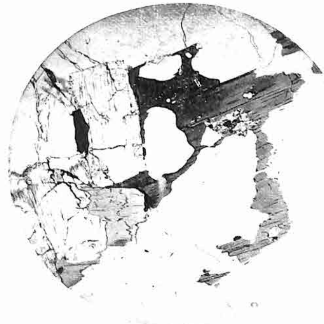
Fig. 6. Corroded 10% biotite crystal in biotite granite. \times 11 , (X. 51).
