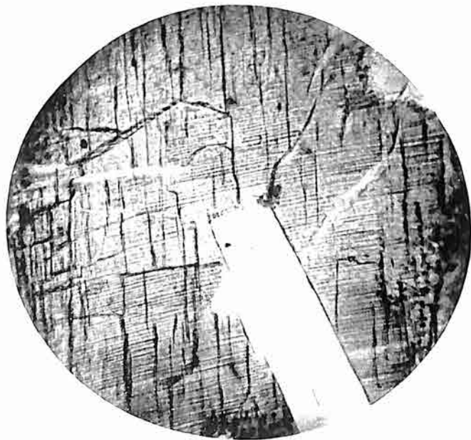
Fig. 3. Coarse (110)-cleavage in monoelinic pyroxene, intersected by fine (001)-cleavage, \times 105 , (Y, 216).
