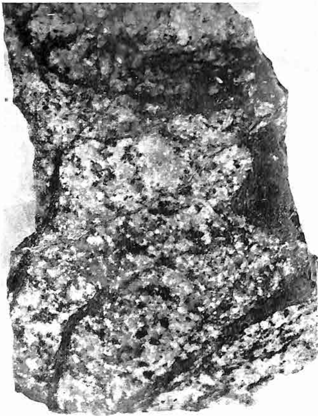
Fig. 3. Pseudotachylyte (black) intruding into biotite granite-gneiss, Coppemano river. (V. 2339).
