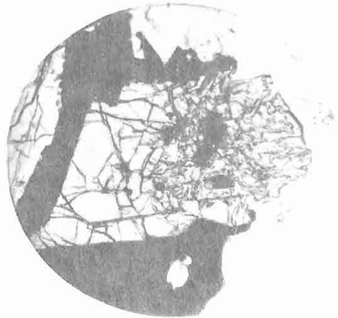
Primary epidote, corroded, in quartz mica hornblende diorite; \times 70 .
