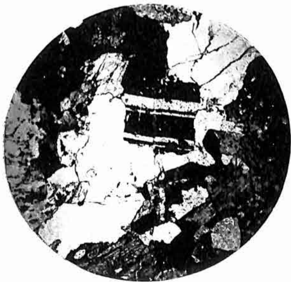
Fig. 5. Idiomorphic plagioclase in hornblende gneiss (ortho-gneiss). Crossed Nicols. \times 16 . (V, 181).
