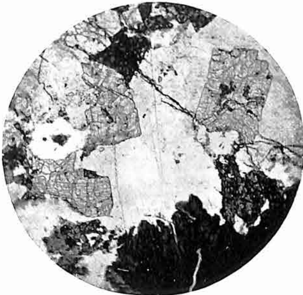
Fig. 3. Idiomorphic topaz and chlorite (dark) in albitite (V. 1065).
