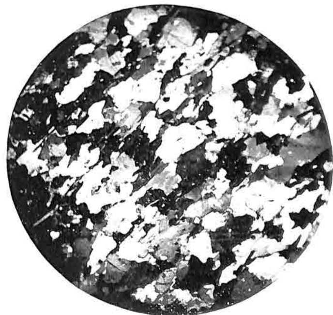
Fig. 6. Quartz mica diorite-gneiss, Crossed Nicols. \times 10 . (V, 208).
