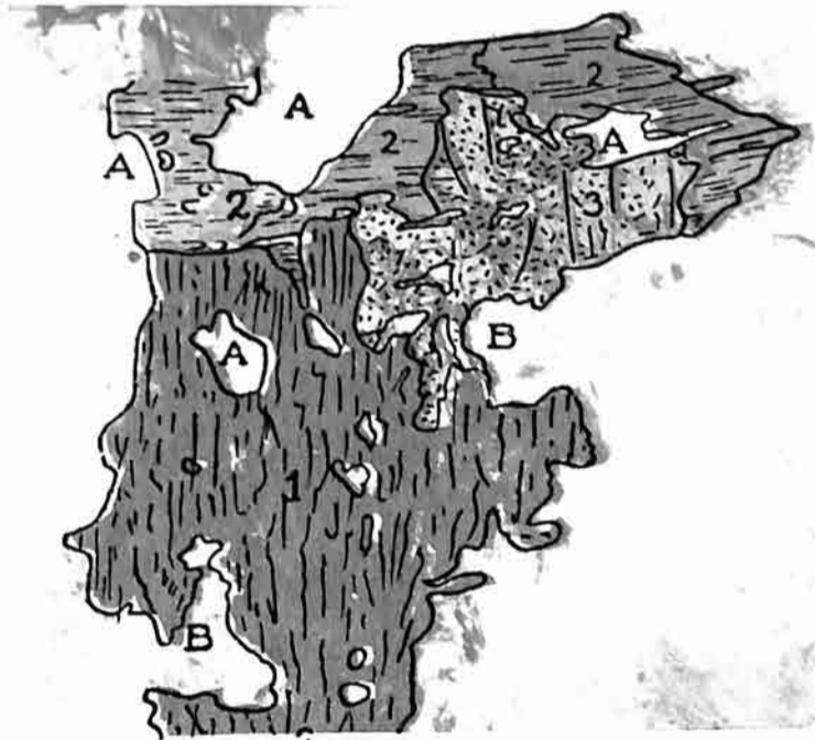
Fig. 3. Group of corroded hornblende, biotite and primary epidote in gneissic diorite, \times 30 , (Y, 14).
