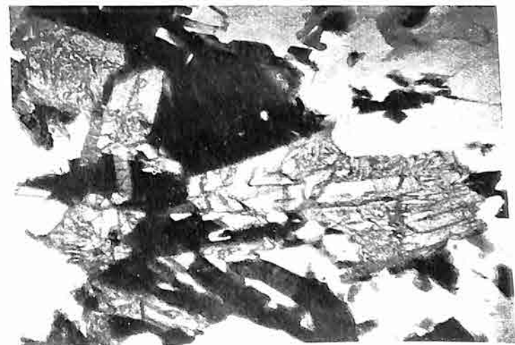
Fig. 6. Idiomorphic primary amphibole enclosed in biotite. diorite-gneiss. \times 51 . (Y. 39).
