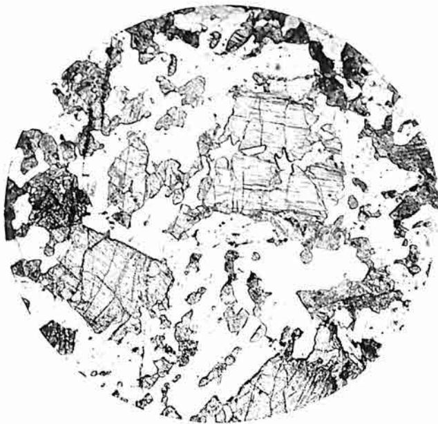
Fig. 3. Pyroxenes of irregular shape in gabbro. \times 13 . (V. 512).
