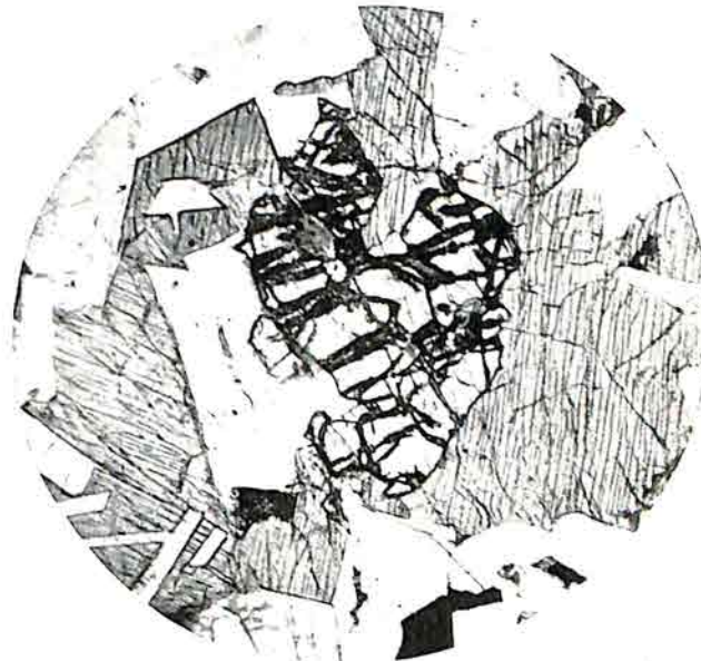
Fig. 4. Olivine replaced by biotite (initial stage). Olivine diabase. \times 48 . (V. 1702).
