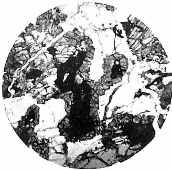
Fig. 3. Reaction-rim of garnet around ore; in gabbro, \times 20 , (V, 2082).
